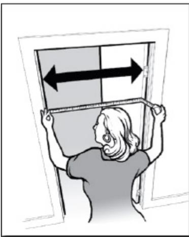
**Measuring the clear opening from the face of the doorstop on the frame to the face of the open door**
