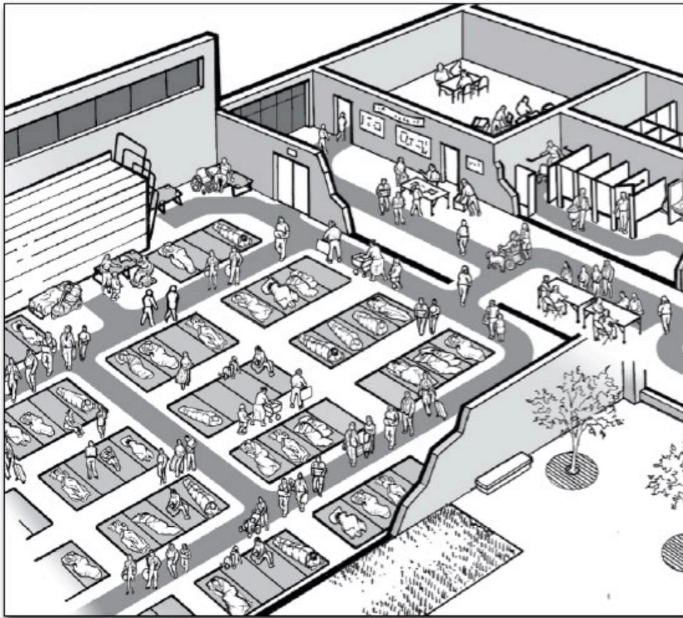
**Interior of one section of a shelter's sleeping area. The shaded pathway indicates the accessible route, which provides access to accessible beds, cots, and other activity areas in the space plus the toilet rooms and other activity areas in the shelter.**
