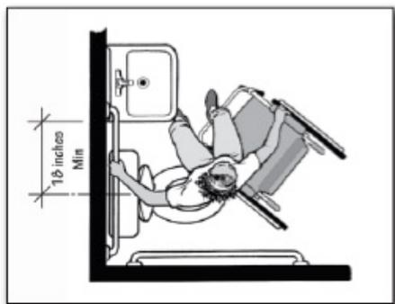
Plan view showing the minimum amount of space required between the toilet and the
