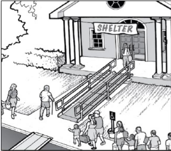
**Three standard parking spaces are converted into an accessible parking space with an access aisle. Cones mark the access aisle and a temporary curb ramp with edge protection connects to an accessible route to the shelter.**
