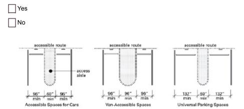
Accessible Parking Spaces Showing Minimum Width of Vehicle Space and Access Aisle
