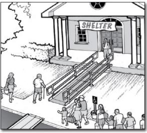
Three standard parking spaces are converted into an accessible parking space with an access aisle. Cones mark the access aisle and a temporary curb ramp with edge protection connects to an accessible route to the shelter.
