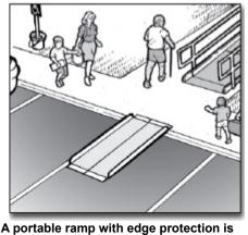
A portable ramp with edge protection is installed over a curb to provide an accessible route.
