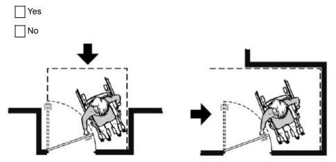
A clear floor space on the latch side of the door (pull side) allows a person using a wheelchair or scooter to pull the door open and then enter. The size of the clear floor spacevaries depending on the direction of approach (shown by the arrows) and the door swing.
