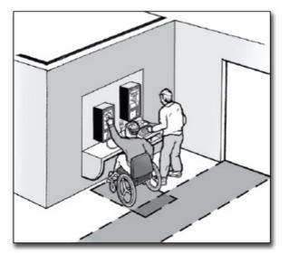
A bank of two public telephones. The accessible telephone is on the left and the telephone on the right is equipped with a TTY.
