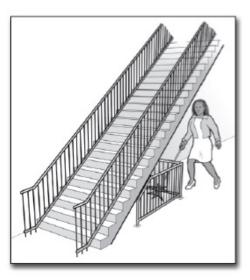
When the underside of a stair is open, it is a hazard to people who are blind or have low vision. Enclosing the area below the stair or installing a cane detectable barrier helps the person to avoid the area.
