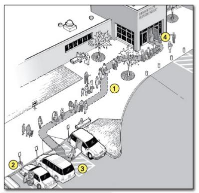
An accessible entrance to a shelter with accessible parking and an accessible drop-off area
